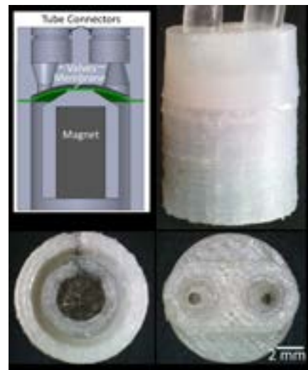
▲ Figure 2: Clockwise from top left: CAD model cross-section of pump; side view of printed pump; top view of printed pump; bottom view of printed pump showing the printed magnet. The scale bar applies to all printed objects.
