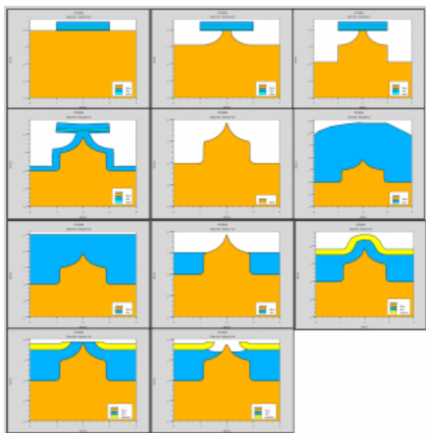
Figure 1: Process flow of the single-gated field emission device, simulated using Silvaco.
