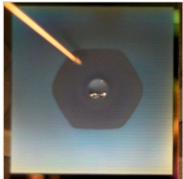
Figure 2: Photograph of fluid being transported through the micropillar patterned surface. Several different spreading regimes can be achieved by varying micropillar geometry.
